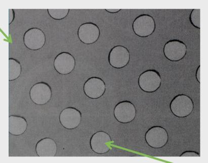
1μm holes with thin layer of amorphous ice
